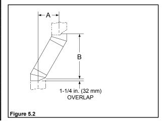
**Example:** Your "A" dimension from Figure 5.2 is 14 1/2 in. (368 mm). Using Table 5.2 the dimension closest to, but not less than 14 1/2 in. (368 mm) is 15 3/4 in. (400 mm) using a 30° offset/return. It is then determined from the table that you would need 36 5/8 in. (930 mm) (Dimension "B") between the offset and return. The chimney components that best fit your application are two SL1112s or SL412s.
